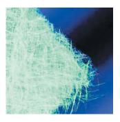
**FARBGLAS 2" filter mats** consists of a spun glass-fibre fabric with compression on the pure-air side, the glass-fibre medium has no wetting agent and is odourless, non-inflammable, and insensitive to moisture in the air
