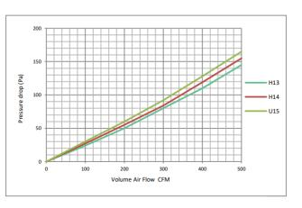
Pressure drop diagram valid for size 592 mm x 592 mm
