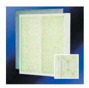
**ULTRANGLAS/ULTRANGLAS-H filter cells** consist of tightly intermeshed glass fibres. ULTRANGLAS is framed on two sides in a moisture-resistant carton frame with large perforation in the metal support plates. ULTRANGLAS / -H is framed on all sides in expanded aluminium mesh and is designed for operating temperatures up to 300°C.
