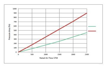
Pressure drop diagram valid for size 592 mm x 592 mm
